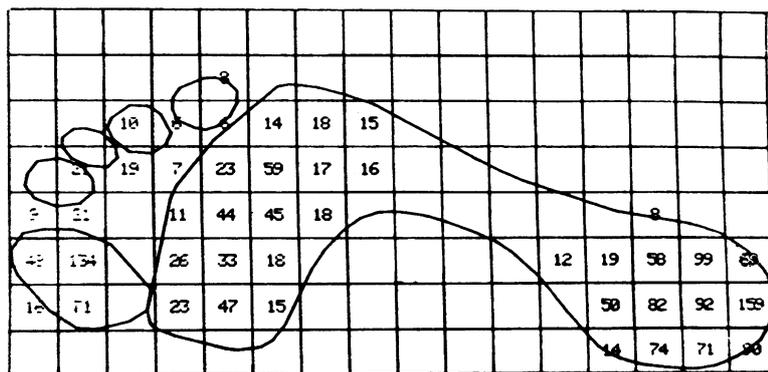
Fig. 3 A computer printout showing the peak forces (in Newtons) exerted on each load cell. The foot outline is shown in correct register.
