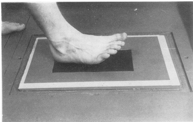
Fig. 2 The walkway with a foot striking the load cells
