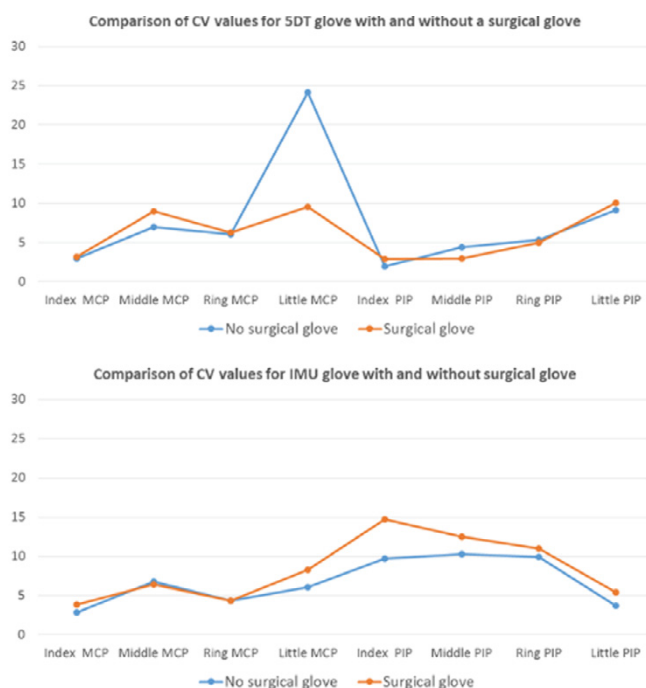
Figure 1: Comparison of Coefficient of Variation (CV) values for mean angular readings for both data gloves, with and without a surgical glove worn underneath.
